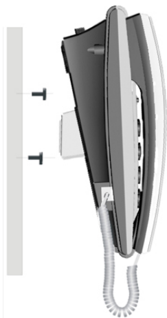
Figure 4-16 FWT vertical placement
