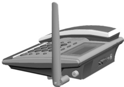
Figure 4-6 Installing an indoor antenna for the FWT
